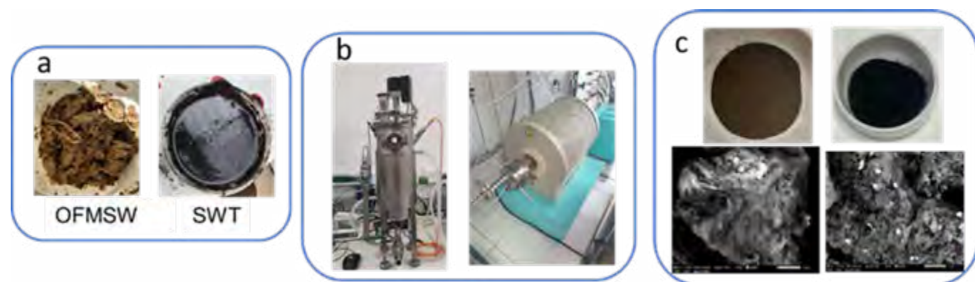
Figure 1. Facilities and materials studied: a) photographs of the wastes selected; b) 5L reactor and oven; c) digestate and carbonaceous materials obtained and corresponding SEM micrographs of the solids.
